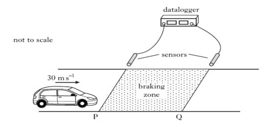
The sensors are connected to a datalogger which records the speed of a car at both P and Q.
